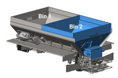
The MultApplier™ allows for two separate materials to be spread simultaneously and features a 24-inch wide #4 belt-over-chain conveyor with 409 stainless steel links. The direct-driven conveyor is also controlled independently enabling the delivery of material at variable rates through the adjustable gate at the rear of the hopper body. The hillside divider improves material placement on the spinner for a more effective spread pattern.
