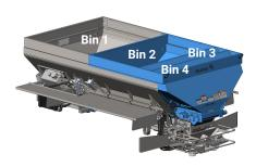
Inserting the MultiBin will convert the spreader to 4 bins, which can be used independently or together for straight and variable rate applications. Sensors are located in all bins to warn when materials are low. The MultiBin also comes equipped with an upper and lower material divider which improves material placement on the spinner for a more effective spread pattern.
