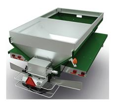
The MultApplier™ allows for two separate materials to be spread simultaneously and features a 24-inch wide #4 belt-over-chain conveyor. The direct-driven conveyor is also controlled independently enabling the delivery of material at variable rates through the adjustable gate at the rear of the hopper body. The hillside divider improves material placement on the spinner for a more effective spread pattern.
