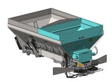
The MultApplier<sup>TM</sup> allows for two separate materials to be spread simultaneously and features a 24-inch wide #4 belt-over-chain conveyor with 409 stainless steel links. The direct-driven conveyor is also controlled independently enabling the delivery of material at variable rates through the adjustable gate at the rear of the hopper body. The hillside divider improves material placement on the spinner for a more effective spread pattern.
