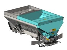
Inserting the MultiBin will convert the spreader to 4 bins, which can be used independently or together for straight and variable rate applications. Sensors are located in all bins to warn when materials are low. The MultiBin also comes equipped with an upper and lower material divider which improves material placement on the spinner for a more effective spread pattern.
