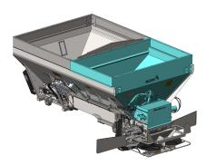
The MultApplier™ allows for two separate materials to be spread simultaneously and features a 24-inch wide #4 belt-over-chain conveyor with 409 stainless steel links. The direct-driven conveyor is also controlled independently enabling the delivery of material at variable rates through the adjustable gate at the rear of the hopper body. The hillside divider improves material placement on the spinner for a more effective spread pattern.
