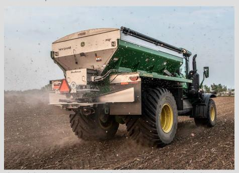
The single bin does not come equipped with the Common Hydraulic Implement Pump on the 800R chassis. The secondary pump is required for the MultApplier, Multibin, and combo machine options.
