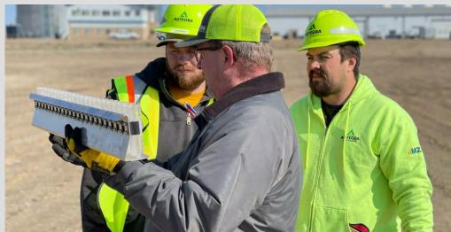
Spread patterns are affected by a number of factors such as type of material being spread, spinner speed, condition of the spinner fins, driving centers, wind and humidity, and rate of material delivery. This makes it critical to perform a spread pattern test in order to make any necessary adjustments.
