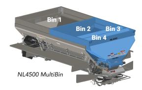
Inserting the MultiBin will convert the spreader to 3 or 4 bins, which can be used independently or together for straight and variable rate applications. Sensors are located in all bins to warn when materials are low. The MultiBin also comes equipped with an upper and lower material divider which improves material placement on the spinner for a more effective spread pattern.
