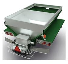
The MultApplier<sup>™</sup> allows for two seperate materials to be spread simultaneously and features a 24-inch wide #4 belt-over-chain conveyor. The direct-driven conveyor is also controlled independently enabling the delivery of material at variable rates through the adjustable gate at the rear of the hopper body. The hillside divider improves material placement on the spinner for a more effective spread pattern.
