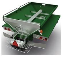
The single bin is available in 304 stainless steel or 409 painted stainless steel. A removable end gate, inverted V, and electric oiler are included. At 15 mph, the single bin can spread fertilizer at rates as high as 1,100 lbs per acre. Add the High Performance option and spread lime at rates as high as 2994 kg (6600 lb) per acre.
