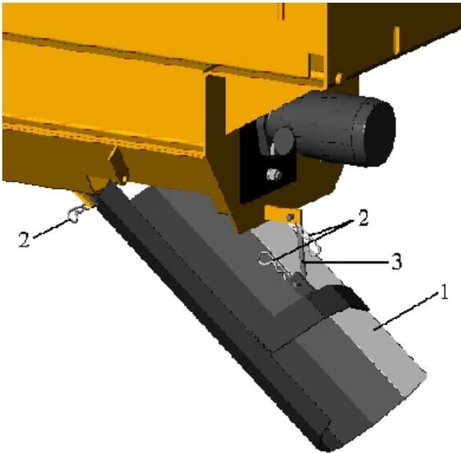
Figure 8 – Berm Chute Installation
