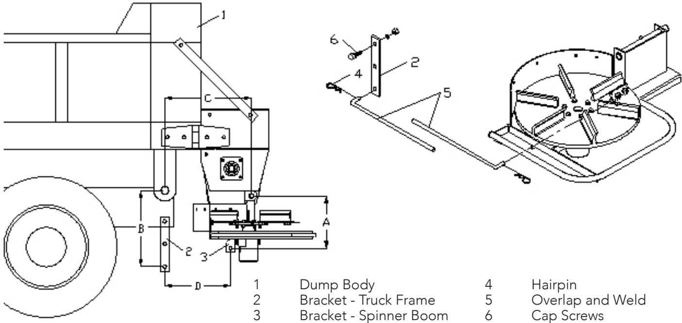
Figure 7 - Leveling Mechanism
