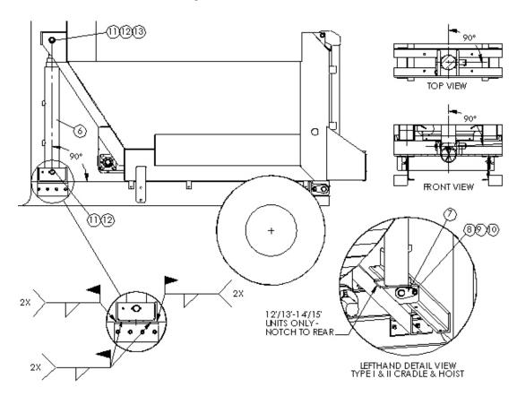
Figure 6 – Hoist Cylinder Installation
