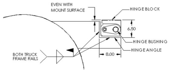
Figure 1 – Hinge Installation
