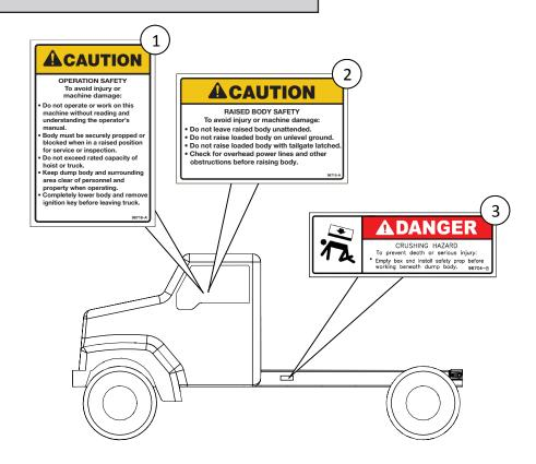
NOTE: Apply decals 1 and 2 in a conspicuous location in the cab of the truck. Apply Decal 3 in a conspicuous location the truck frame, behind the cab.
