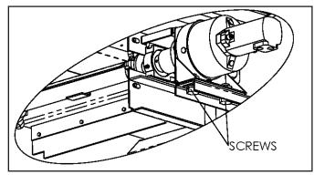
Figure 2 - Gear Case Mounting Bolts
