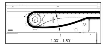
Figure 4 - Cross Conveyor Chain Tension
