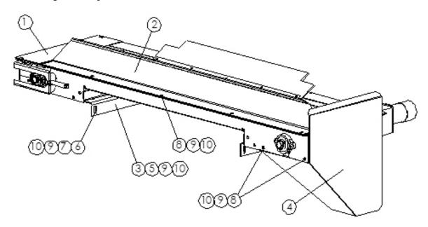
Figure 7 – Cross Conveyor Assembly
