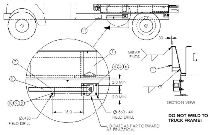
Figure 4 – Body Prop Installation
