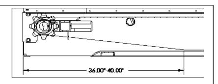
Figure 3 - Main Conveyor Chain Tension
