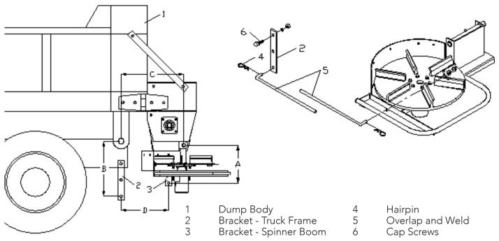
Figure 7 - Leveling Mechanism
