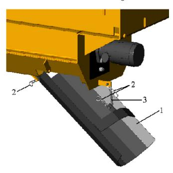
Figure 8 – Berm Chute Installation
