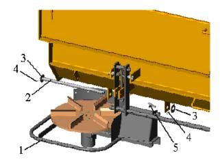
Figure 5 – Spinner Installation
