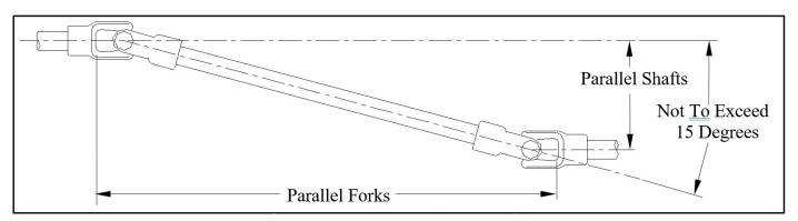
Figure 1 - Timing of Universal Joints
