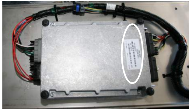
Figure 54 - Dry Rate Controller Serial Tag (Located under frame towards front of unit.)
