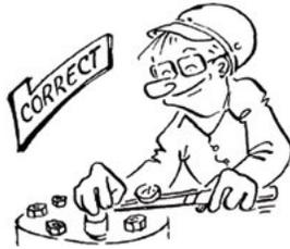
13. Shut off engine before filling fuel and oil tanks. Do not allow overflow. Wipe up all spills. Do not smoke. Stay away from open flame. FIRE HAZARD!
