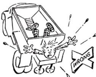
5. Guards and covers are provided to help avoid injury. Stop all machinery before removing them. Replace guards and covers before starting spreader operation.
