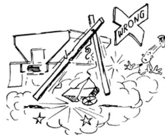
8. If repairs require use of a torch or electric welder, be sure that all flammable and combustible materials are removed. Fuel or oil reservoirs must be emptied, steam cleaned and filled with water before attempting to cut or weld them. **DO NOT** weld or flame cut on any tank containing oil, gasoline or their fumes or other flammable material, or any container whose contents or previous contents are unknown.
