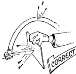
14. The fine spray from a small hydraulic oil leak can be highly explosive—**DO NOT SMOKE**—**STAY AWAY FROM FLAME OR SPARKS**.
