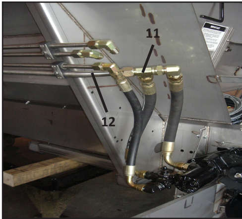
Figure 12D – LH Hydraulics at Rear Existing
