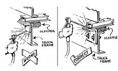
and must be avoided. When drilling holes in frame member, drill only through the vertical web portions do not put holes in top or bottom flanges. Refer to truck manufacturer's recommendations.
