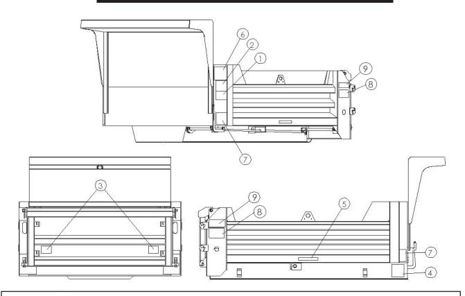
Install "Danger - Crushing Hazard" decals (PN 96704) on front of both truck frame rails, in IMPORTANT! clear view. Install "Caution – Operation Safety" (PN 96716) and "Caution – Raised Body" (PN 96715) decals in clear view in truck cab.
