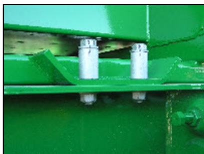
Figure 12b – Center Mounts (2nd) 315 ft-lb (425 nm) torque
