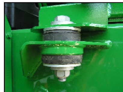
Figure 12c – Front Mounts (3rd) 315 ft-lb (425 nm) torque
