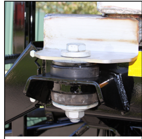
Figure 3c – Front Mounts (3rd) 330 ft-lb (450 nm) torque
