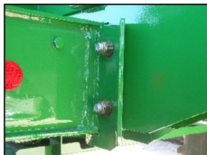
Figure 12a – Rear Mounts (1st) 315 ft-lb (425 nm) torque
