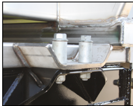
Figure 3b – Center Mounts (2nd) 234 ft-lb (315 nm) torque
