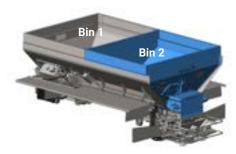
The MultApplier™ allows for two separate materials to be spread simultaneously and features a 24-inch wide #4 belt-over-chain conveyor with 409 stainless steel links. The direct-driven conveyor is also controlled independently enabling the delivery of material at variable rates through the adjustable gate at the rear of the hopper body. The hillside divider improves material placement on the spinner for a more effective spread pattern.
