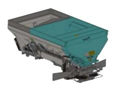
Inserting the MultiBin will convert the spreader to 4 bins, which can be used independently or together for straight and variable rate applications. Sensors are located in all bins to warn when materials are low. The MultiBin also comes equipped with an upper and lower material divider which improves material placement on the spinner for a more effective spread pattern.
