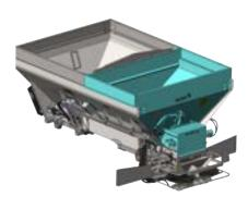
The MultApplier™ allows for two separate materials to be spread simultaneously and features a 24-inch wide #4 belt-over-chain conveyor with 409 stainless steel links. The direct-driven conveyor is also controlled independently enabling the delivery of material at variable rates through the adjustable gate at the rear of the hopper body. The hillside divider improves material placement on the spinner for a more effective spread pattern.
