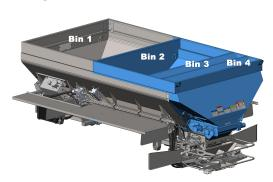
Inserting the MultiBin will convert the spreader to 3 or 4 bins, which can be used independently or together for straight and variable rate applications. Sensors are located in all bins to warn when materials are low. The MultiBin also comes equipped with an upper and lower material divider which improves material placement on the spinner for a more effective spread pattern.
