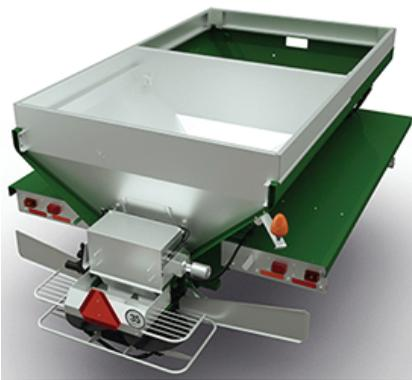
The Multiplier™ allows for two separate materials to be spread simultaneously and features a 24-inch wide #4 belt-over-chain conveyor. The direct-driven conveyor is also controlled independently enabling the delivery of material at variable rates through the adjustable gate at the rear of the hopper body. The hillside divider improves material placement on the spinner for a more effective spread pattern.
