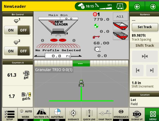
The 800R series utilizes the **4600 CommandCenter** but with tailored functions to meet the needs of operators. All key functions are visible in one screen.
