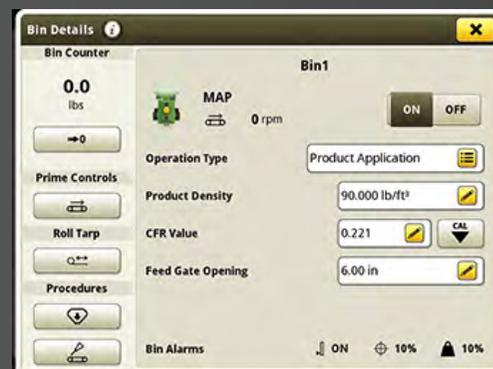
The **Bin Details** page provides users with more frequent dry spinner spreader inputs and adjustments. For dry spinner spreaders with multiple bins, individual tabs at the top of the screen make it easy to quickly toggle between them.
