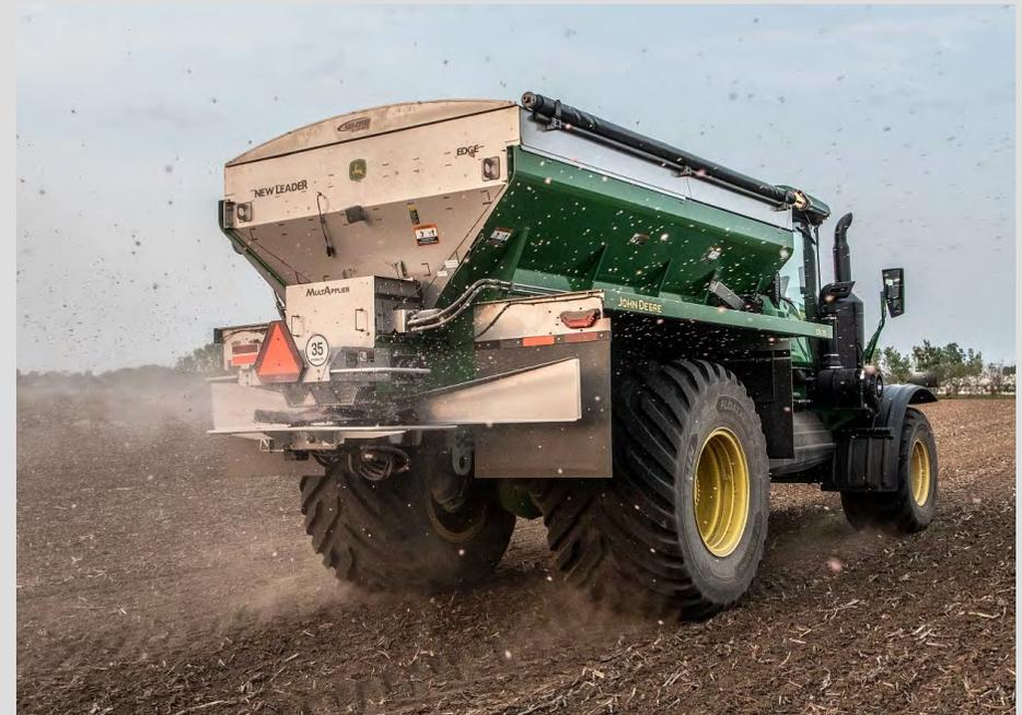
The single bin does not come equipped with the Common Hydraulic Implement Pump on the 800R chassis. The secondary pump is required for the MultiApplier, Multibin, and combo machine options.
