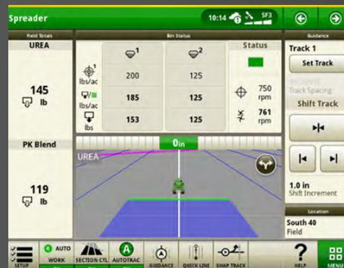
The **SpreadStar** control system provides superior rate control, response times, and ease of use. All key functions are on one display screen in the cab of your machine for complete machine control and monitoring in one simple, easy-to-use package.
